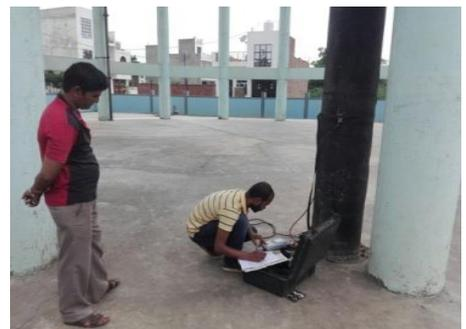
As seen in field activity & flow measurement, the average flow rate of Inlet is 281.26 m<sup>3</sup>/ hr. and hence total Inlet to Kalandi vihar OHT is 3.37 MLD.
