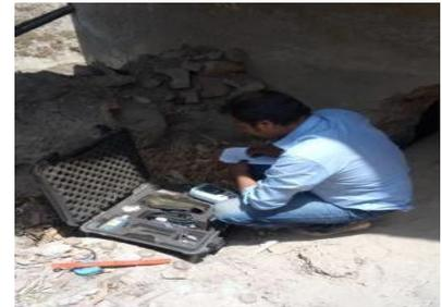
As seen in flow mesurment activity, the average flow to Jeoni Mandi WTP from Raw water New intake well 1976.6 m3/hr and hence Inlet Supply to WTP is 21.59MLD.
